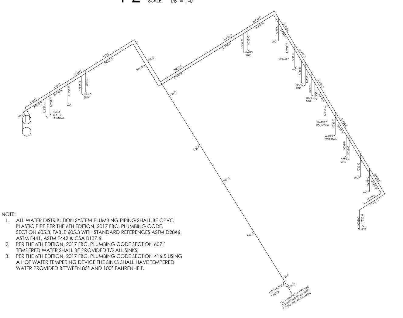
PROPOSED POTABLE WATER PLUMBING SCHEMATIC
